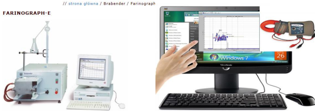
Fig. 1 a: Brabender farinograph; b: Portable device for measuring the consumed current at the kneading arm
